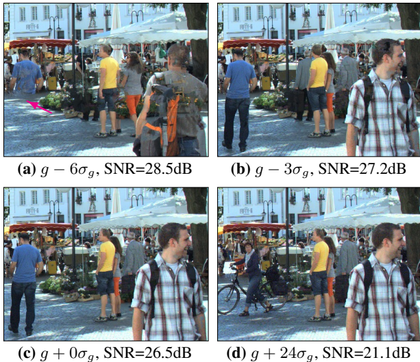
Figure 5: Sensitivity of our deghosting method to gain calibration accuracy. Here, g , \sigma_g denote the mean and standard deviation of the flat-field gain calibration. Our method is robust to slight under-estimation (b) and large over-estimation (d) of the camera gain: When it is under-estimated (which occurs seldom, see Fig. 4), ghosting artifacts can appear (a, magenta arrow). Conversely, when the gain is over-estimated, it leads to low SNR (d), but it does not introduce ghosting artifacts. See supplementary material for additional tests at intermediate error levels.
