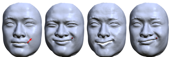
Figure 8: Results of direct manipulation of the underlying basis. From left: user-constraints, PCA basis, Varimax Basis, Our basis. PCA effects unintuitive global deformation even if the edits are local. Varimax basis shows artifacts. Ours provides artistically meaningful local edits.
