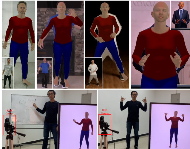
Figure 1: We present the first real-time monocular approach that jointly captures shape and pose of body and hands together with facial geometry and color. Top: results on in-the-wild sequences. Bottom: real-time demo. Our approach predicts facial color while the body color is set manually.
