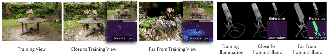
Fig. 1. We propose a method to quantify uncertainty in radiance fields using a novel and efficient manifold sampling strategy. Our approach allows for differentiable optimization of views to reduce reconstruction ambiguities. We demonstrate this capability in next-best view planning (left) and illumination planning (right) tasks.
