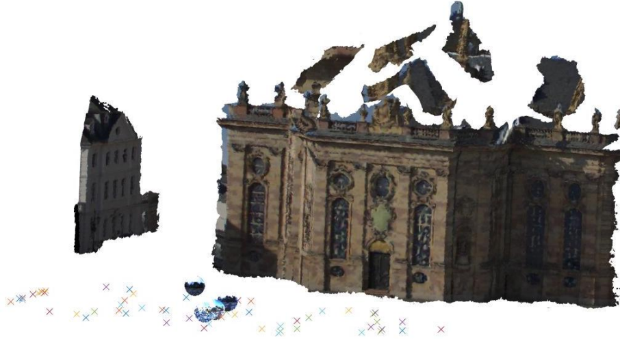
Fig. 10: Reconstructed scene used in our benchmark. Estimated camera positions are shown as crosses and the aligned environment maps rendered on spheres.
