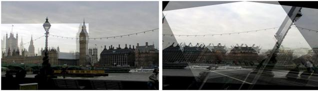
**Figure 20:** Left: Ghosting on static objects such as Big Ben. Right: Significant skewing in a considerable view change transition.
