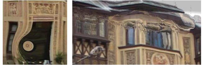
**Figure 18:** Artifacts in the warp transitions, taken as zoomed regions of Figure 17. Left: Swirl artifacts from incorrect feature point correspondence. Here, a feature to the left of the door has been matched with a feature to the right, causing the warp to generate a swirl. Right: Flickering at the boundary between images, where the flow between the two overlaid images is undefined.
