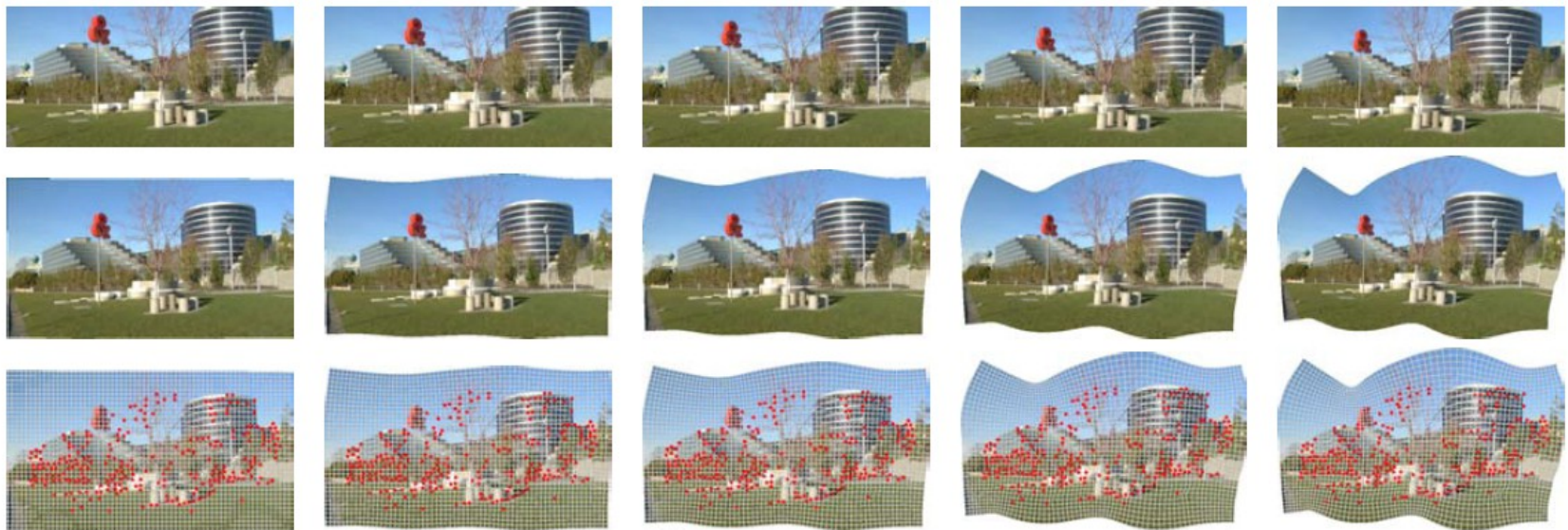
Figure 6: Each row shows a sequence of warps of a single input video frame created by pulling the camera away from its original location. The top row shows the final cropped result; the middle shows the entire warp result; the bottom shows the corresponding grids and the points that guide the warp. For small camera motions the warps look reasonable, but they become visibly distorted at larger camera displacements.
