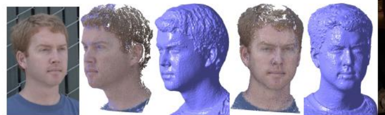
Multi-view stereo reconstruction
